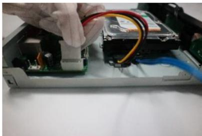
6. Connect the power cable to the motherboard.
