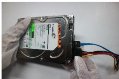
2. Connect one end of the data and power cables to the hard
