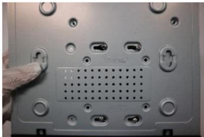
4. Align screws with screw holes on the bottom plate, and then slide the hard disk in position.
