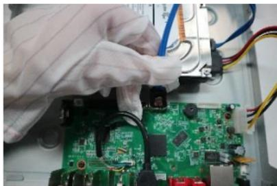
7. Connect the data cable to the motherboard.
